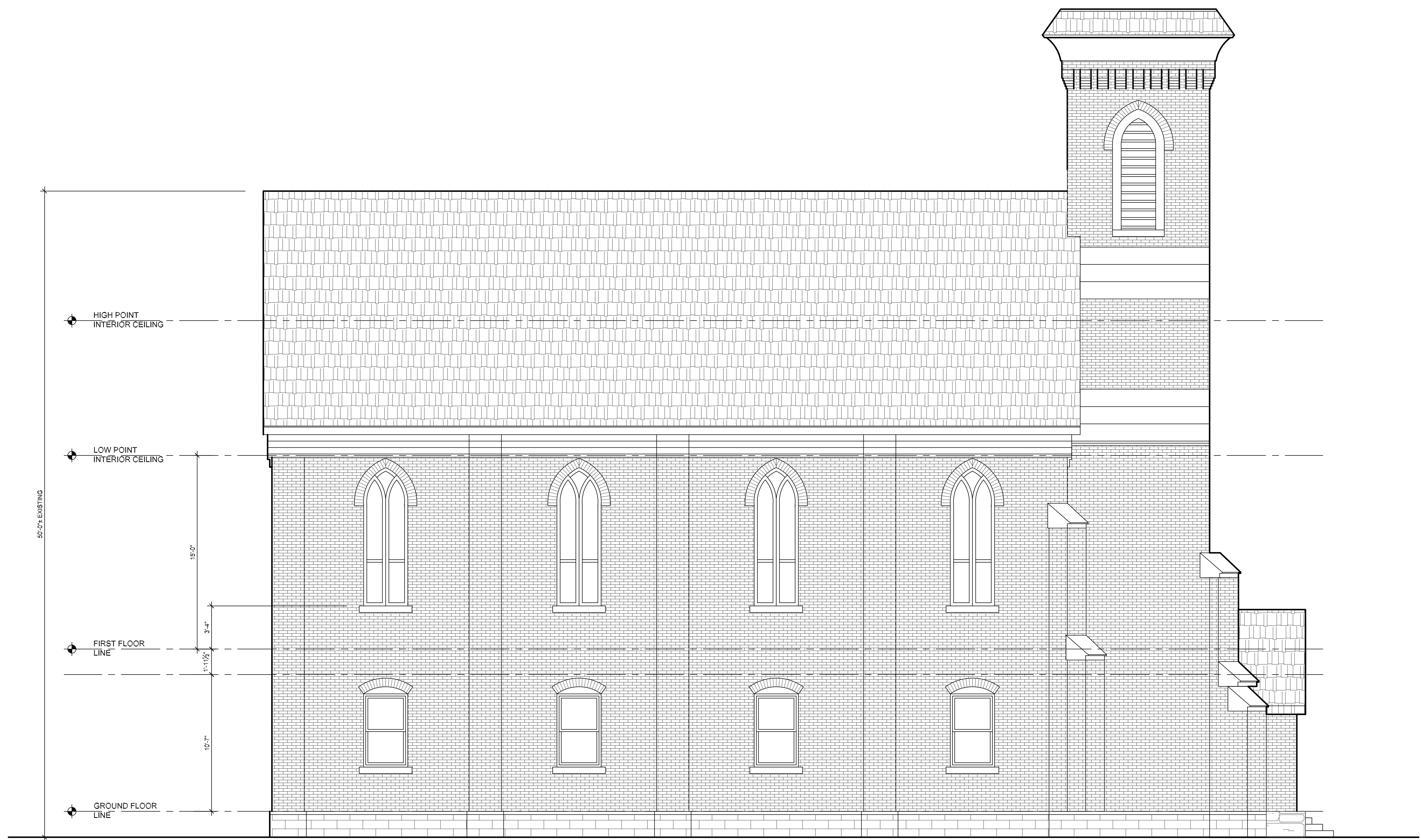
EXISTING SOUTH ELEVATION SCALE: 1/4" = 1'-0"
