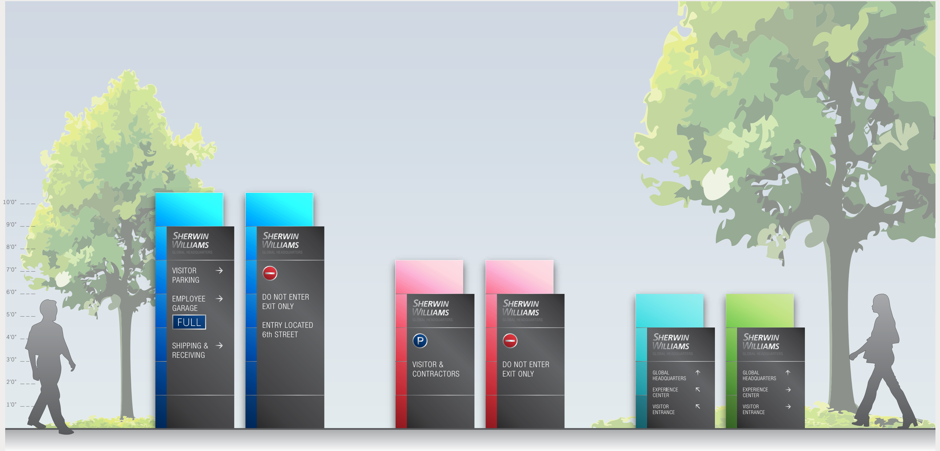
ELEVATION: VEHICULAR & PEDESTRIAN DIRECTIONALS – FRONT SCALE: 3/8" = 1'0"
