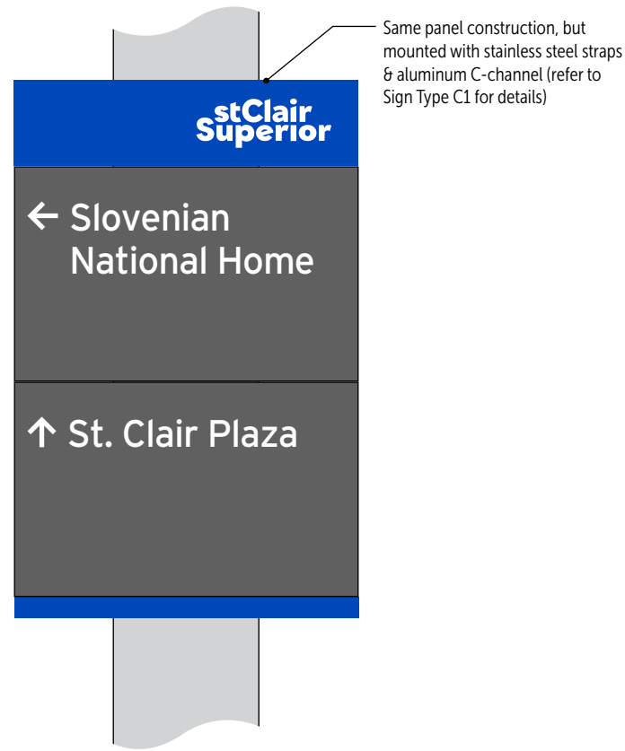
MOUNTED TO EXISTING UTILITY POLE Scale: 1/2" = 1'
